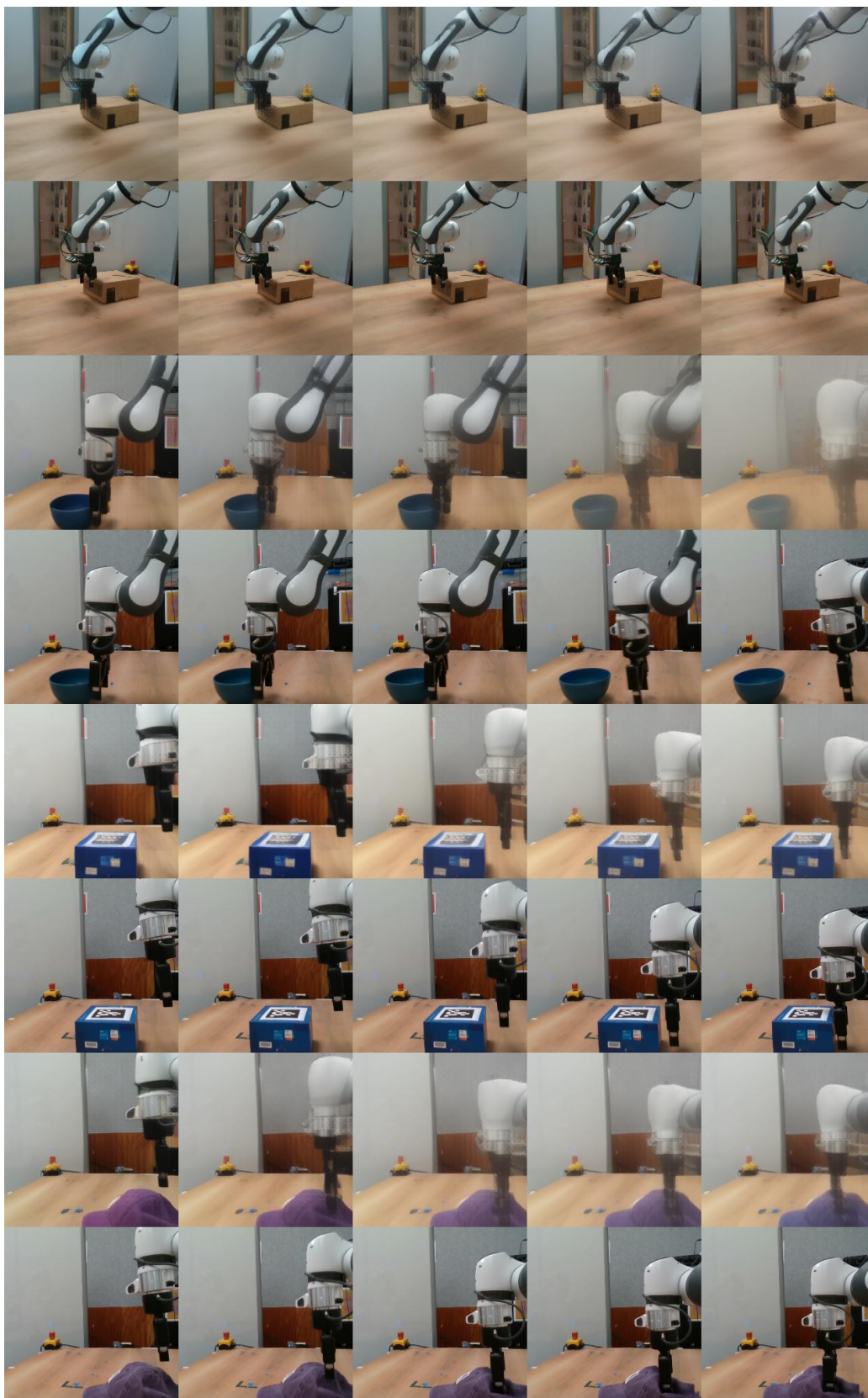
Figure 14: Unrolling a trajectory with our proposed JEPA-WM on some of our collected Franka arm trajectories, with our best model presented in Section 5.3. For each pair of rows, the top one is the model’s visual decoding of the action unrolling, the bottom one is the ground-truth trajectory of the dataset. The model sometimes does not grasp well interaction with objects, which is the most frequent failure case.
